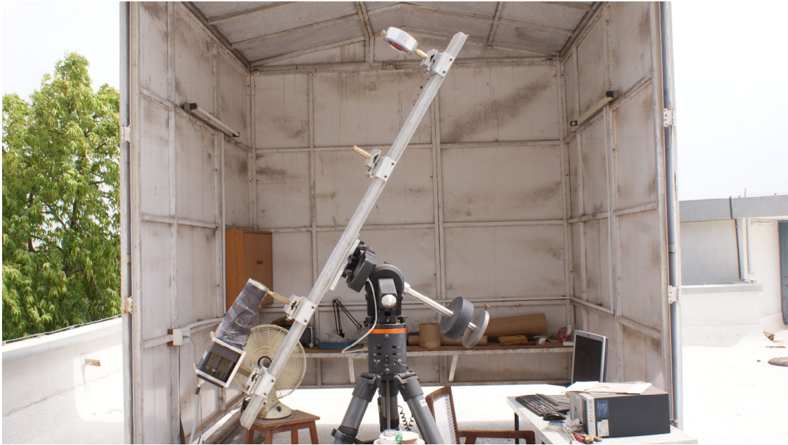
Figure 2: The 100 mm diameter refracting full disk solar flare telescope installed at the terrace of main building at Thaltej campus of PRL, Ahmedabad. The auto-drive telescope is equipped with high quality filters and CCD camera suiting to take solar observations at fast cadence of 100 milliseconds. The images are processed with special software to extract the science information.
