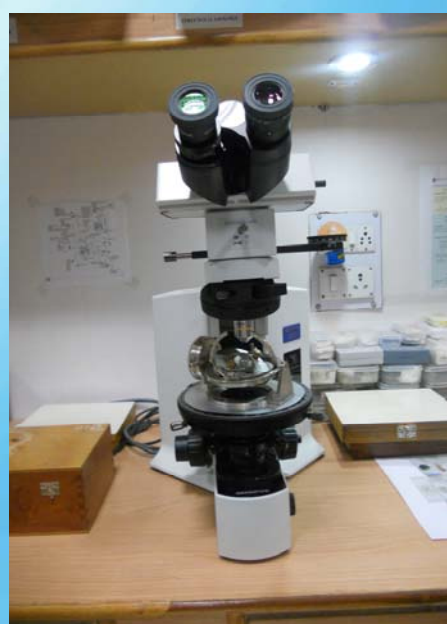
Figure 7. PLANEX facility developed in University of Allahabad for PDFs indexing using 4-axes Universal Stage (kindly donated by Professor Olaf Madenbach, Ruhr University, Germany).
