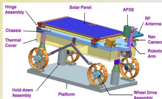
**sub-systems. The position of APXS on the robotic arm is indicated.**
