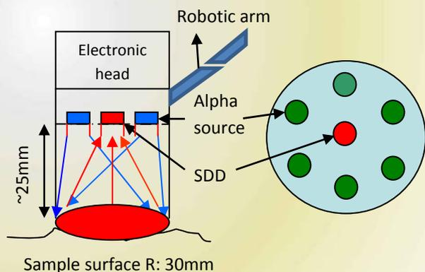
Fig. 2. APXS sensor head
