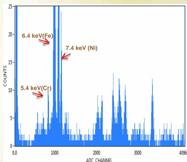
**Fig. 5.** Spectral response obtained from Allende sample with  $^{241}\text{Am}$  source. The peaks and corresponding elements are indicated
