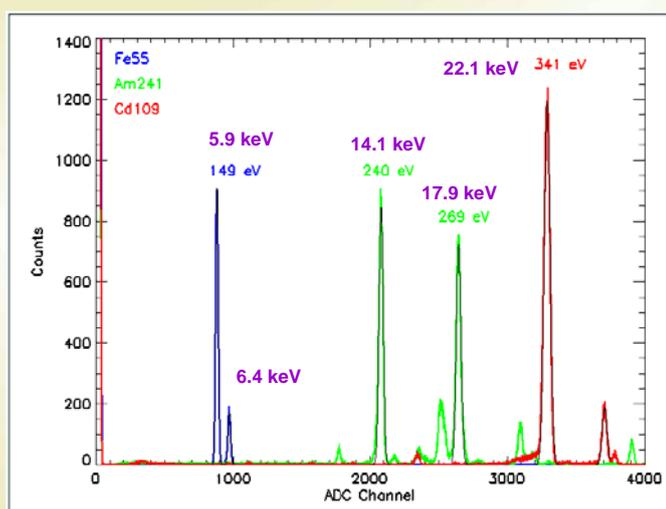
**Fig. 4.** Spectral response obtained using three X-ray sources ( $^{55}\text{Fe}$ ,  $^{241}\text{Am}$  and  $^{109}\text{Cd}$ ). The peak energy [keV] and the FWHM [eV] are indicated
