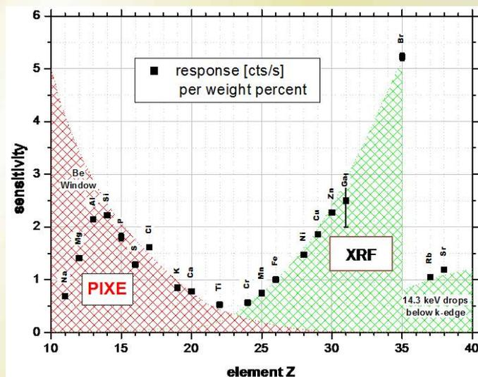
Fig. 3. Sensitivity of X-ray production by PIXE and XRF, as a Function of Z.
