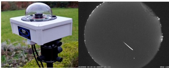
An Image of an All Sky Camera with a captured image
