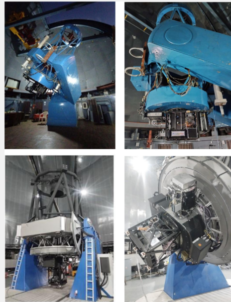
Figure 2: Images showing ProtoPol mounted on PRL 1.2 m (top) and 2.5 m telescopes at Mt. Abu (bottom).
