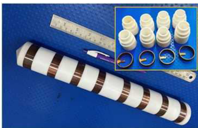
Figure no. 18: PRATHIMA Payload (for Chandrayaan-5/LuPEX mission): Probe Lab Model
