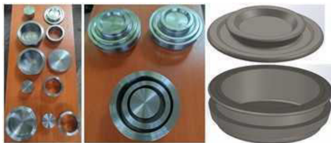
Figure no. 6: Sample Crushing Sets for High-Frequency (vibration) Sample Crusher
