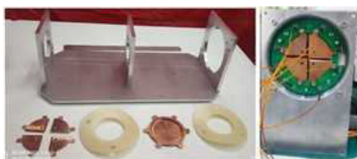
Figure no. 26: DM Payload Testing – Fabrication of Lens System and Copper Detectors
