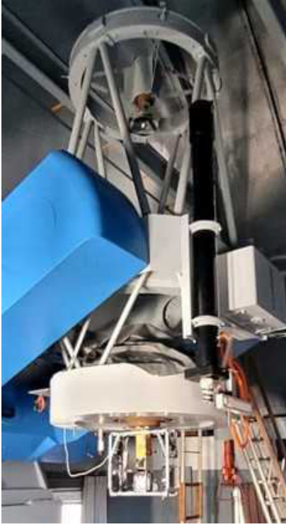
Figure 38 : EMPOL instrument mounted on PRL 1.2m telescope.
