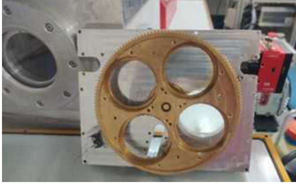
Figure 30 : Four position cryo filter wheel
