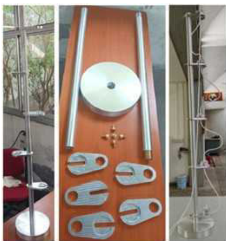
Figure no. 7: In-line Sequential Filtration Unit for Phytoplankton Isolation
