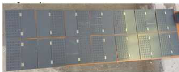
Figure no. 10: Fabrication of PVC Platters with Hinged Covers
