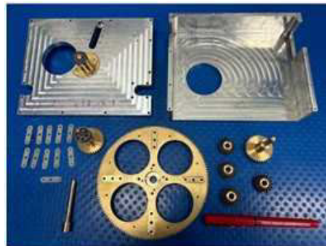
Figure no. 16: NISP: Filter Wheel Assembly for Vacuum Testing
