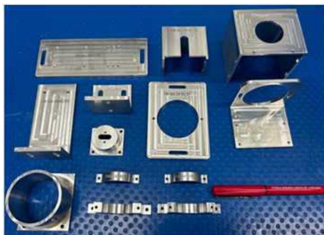
Figure no. 17: Proto-Pol Instrument Parts for Fibre Arrangement in Calibration Unit and Slit Viewer
