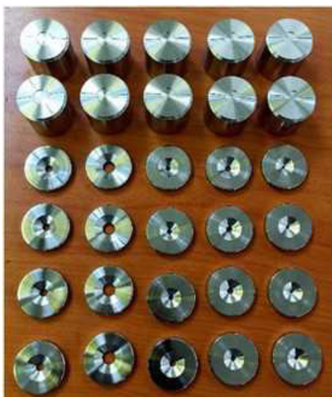
Figure no. 11: SS-304 Sample Holders Base and SS-304 Covers for Samples.
