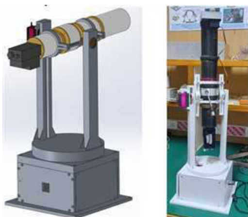
Figure no. 3: Robotic Photometer Assembly (2-Axis Sky Imager)
