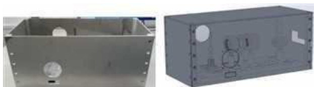
Figure no. 15: Xenon Arc Lamp Assembly for Faint Object Camera (FOC) in PARAS-2 Instrument
