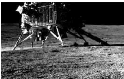
Figure 1: Image of the Vikram lander with ChaSTE probe deployed into the lunar surface
