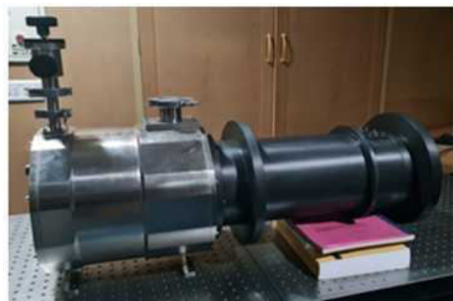
Figure 16 : The PARAS-2 cryogenic dewar in the lab for testing and verifications.
