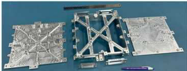
Figure no. 21: DISHA mission- Drift Meter Payload: Power and Processing Electronics Enclosures
