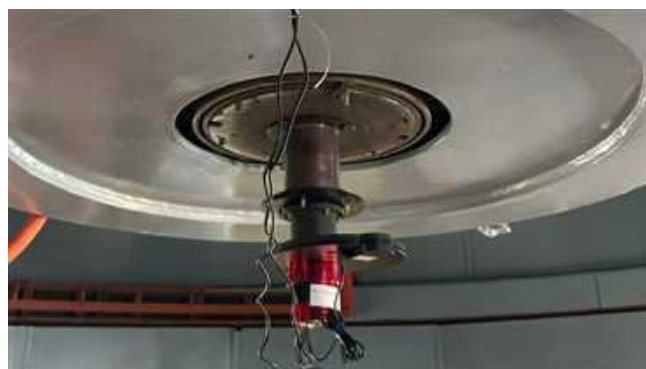
Figure 36 : Imager mounted on the PRL 1.2m telescope at Mt Abu.
