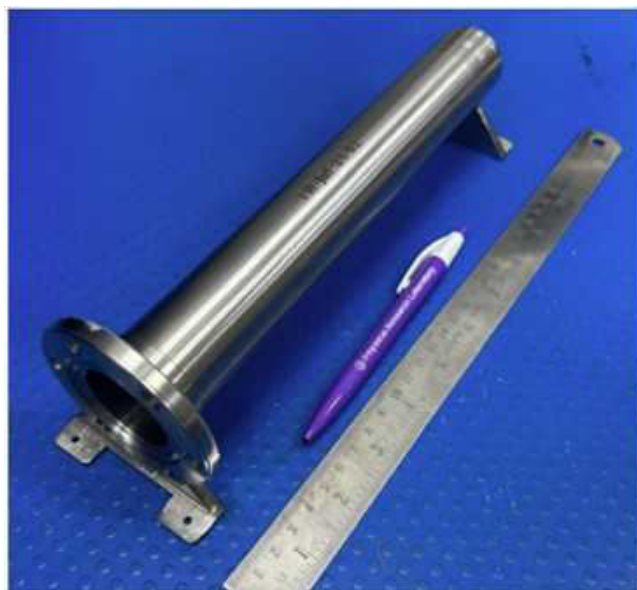
Figure no. 27: Shield Tube for NIMS Instrument for Future Space Science Missions.
