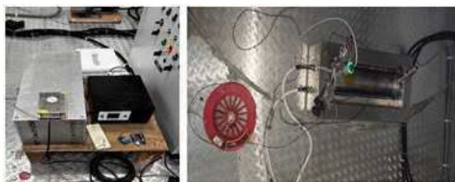
Figure 15 : Left : Xenon arc lamp set up, Right : Fabry-Perot optics inside the vacuum chamber which is kept in a thermally stable water bath.
