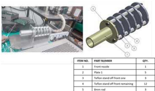
Figure no. 25: Lens System for RPA Sensor Calibration
