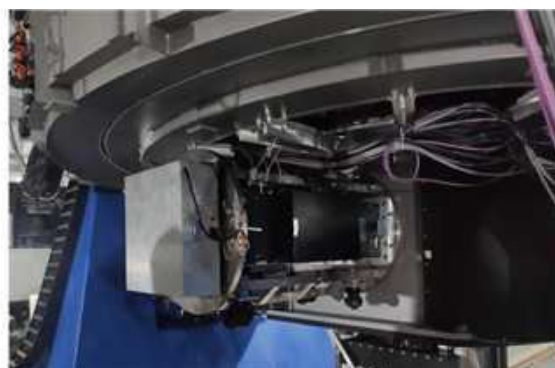
Figure 29 : The Low-Resolution Spectrograph on the side port of the 2.5m telescope.
