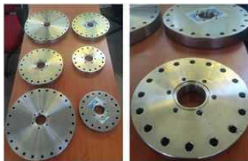
Figure no. 9: Machining of Knife Edges and PCD Tapping on SS-304 CF Flanges - Femtosecond Lab
