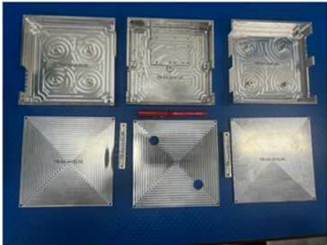
Figure no. 22: DISHA Mission- Langmuir Probe Payload: Electronics Enclosures
