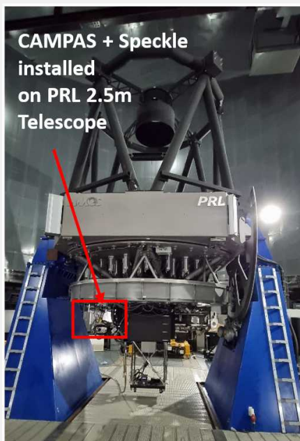
Fig: CAMPAS + Speckle installed on PRL 2.5m Telescope at PRL Mount Abu Observatory.
