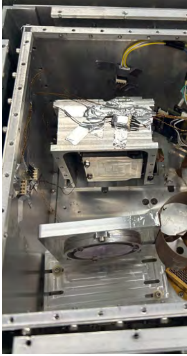
Figure 28: Setup for imaging using H2RG detector with Y Filter.
