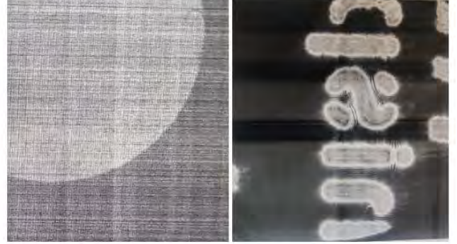
Figure 29: The left panel shows the circular obstruction in the collimated beam. The right panel shows the "nisp" mask cutout in the collimated beam.
