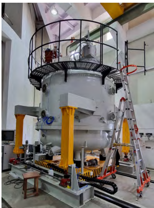
Figure 23: Mirror Coating plant for 2.5m diameter mirror installed at PRL Mount Abu Observatory at Gurushikhar, Mount Abu.
