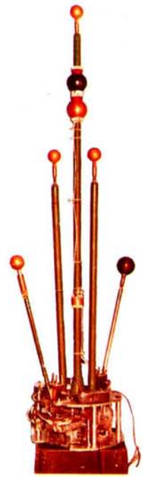
▲ 2.17 (a) Plasma probes for making insitu measurements of plasma parameters like electron density, electron temperature, and ac electric fields have been developed in
