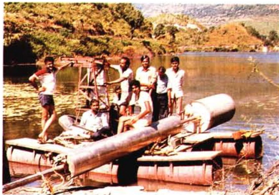
◀ 3.18 Sediment sampling from a Naukuchia Tal lake bottom by means of a 6 m Mackereth corer made at PRL. Recent sediments from lakes are being studied at PRL to infer the characteristics of the depositional environment.
