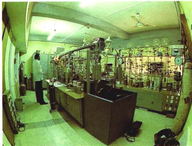
► 3.15 A view of the Radiocarbon Laboratory. The glass vacuum assembly used for purification of carbon dioxide and methane gas was fabricated at PRL.
