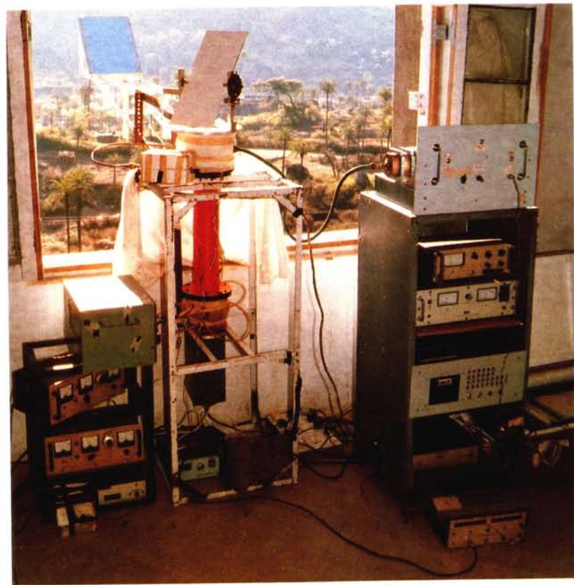
◀ 2.26 A high resolution Fabry-Perot spectrometer for measuring winds and temperatures in the airglow emitting regions.
