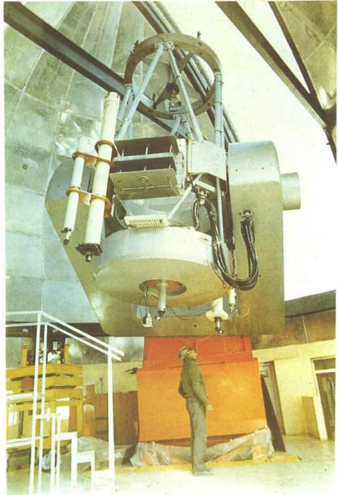
▲ 1.6 1.2 metre aperture telescope for infra-red astronomy established at Gurushikhar peak, Mount Abu (Rajasthan).
