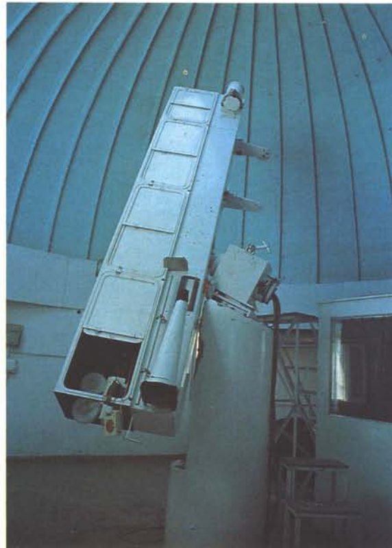
◀ 1.15 (a) The 12 feet spar telescope used at USO for high resolution observations of solar chromosphere.
