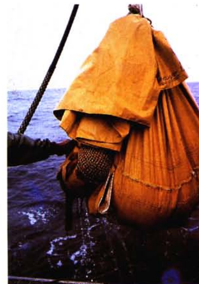
3.8 Si-32 is a radioactive isotope used for determining the rates of large scale ocean circulation. Its measurement requires its extraction from tons of sea water and assay using high sensitive counters. Techniques towards some of these have been developed by PRL scientists. (a) Scientists filling the bag sampler with fibres on the ship's deck. (b) Bag sampler containing chemically coated synthetic fibres for extraction of silica from seawater. (c) Si 32 counting laboratory — the radiation detectors are developed at PRL.
