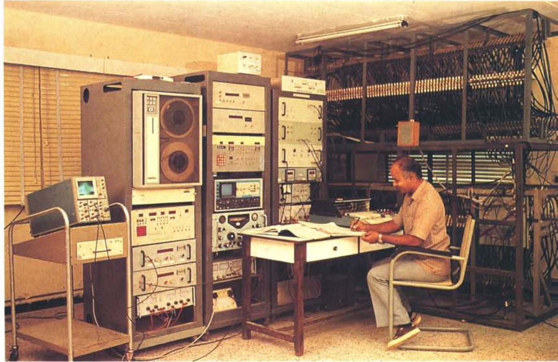
▲ 1.22 (b) Butler Matrix, correlation receiver and the recording system at Thaltej Field Station.
