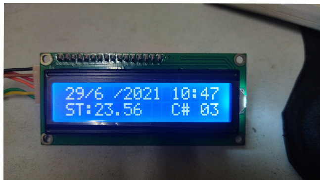
Figure 7. The 16 x 2 LCD unit, displaying the real-time parameters during the working of the Automated Freeze-Thaw instrument
