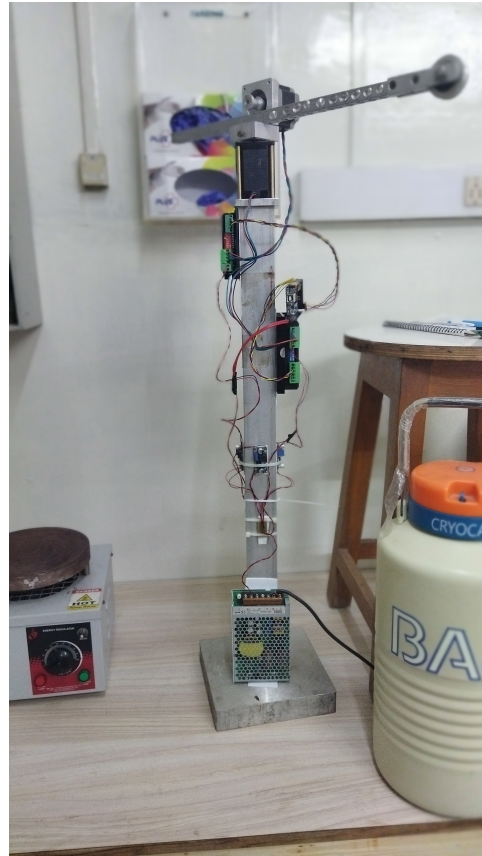
Figure 9. The Automated Freeze-Thaw instrument, after configured mechanically and electronically
