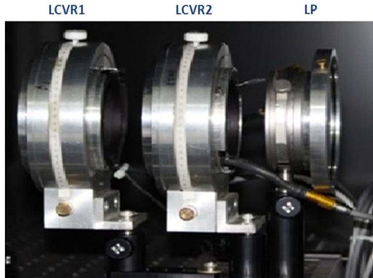
Figure 2 Imaging polarimeter for MAST at USO. From left to right, we show LCVR1, LCVR2, and the linear polarizer. LCVR1 and LCVR2 are kept at 0^\circ and 45^\circ with respect to the linear polarizer (LP), respectively.
