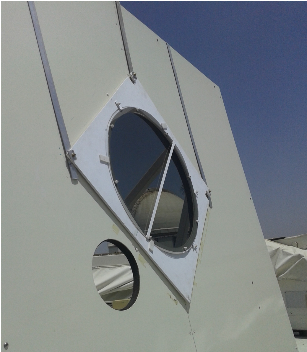
Figure 6.1: Sheet polarizer is placed in a rotating mount on the sunshield of MAST.
