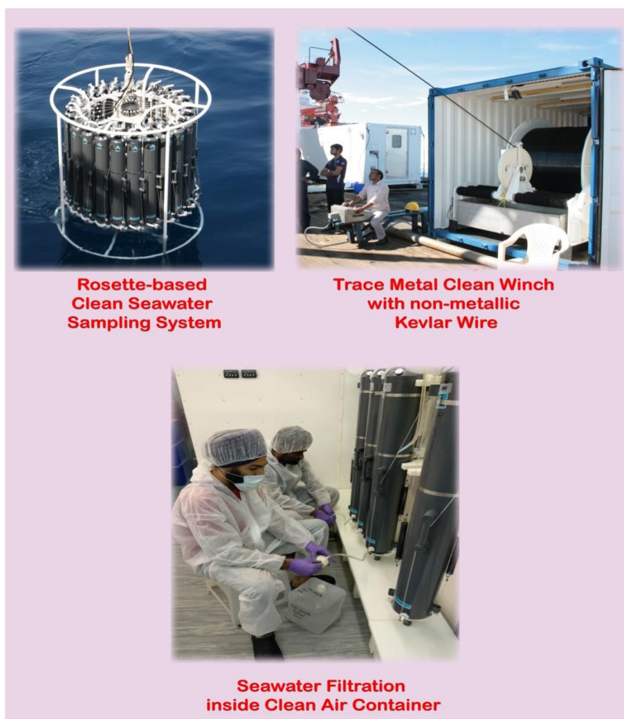
Fig. 2.2: Top: Rosette-based, trace metal clean sampler with 24, 12L Niskin bottles (top left) and clean winch equipped with non-metallic, Kevlar wire (top right). Bottom: Image showing the processes of seawater sample filtration inside the clean air (class 1000) container.
