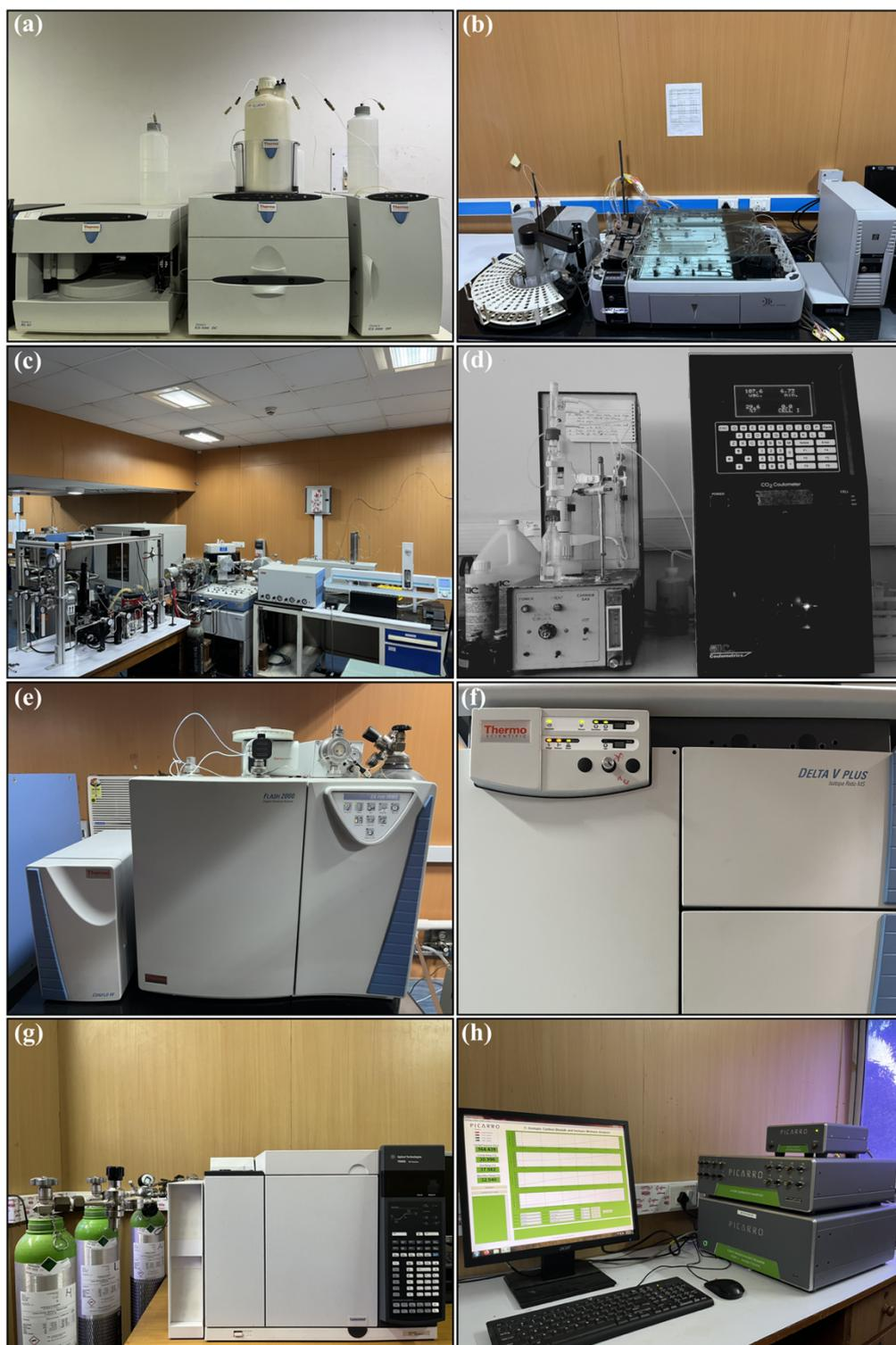
**Fig. 2.2** Picture of the (a) ion chromatography, (b) autoanalyzer, (c) gas bench –IRMS (MAT 253), (d) coulometer, (e) elemental analyzer, (f) IRMS (Delta V Plus), (g) gas chromatography, and (h) cavity ring down spectroscopy (Picarro) at the Physical Research Laboratory (PRL), India. These instruments are regularly used, including for this thesis, to generate data at PRL.
