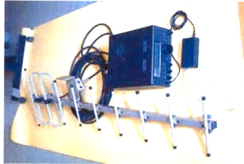
Figure 2.8. Component of the ground instrument setup (Antenna, wide band receiver and Modem).
