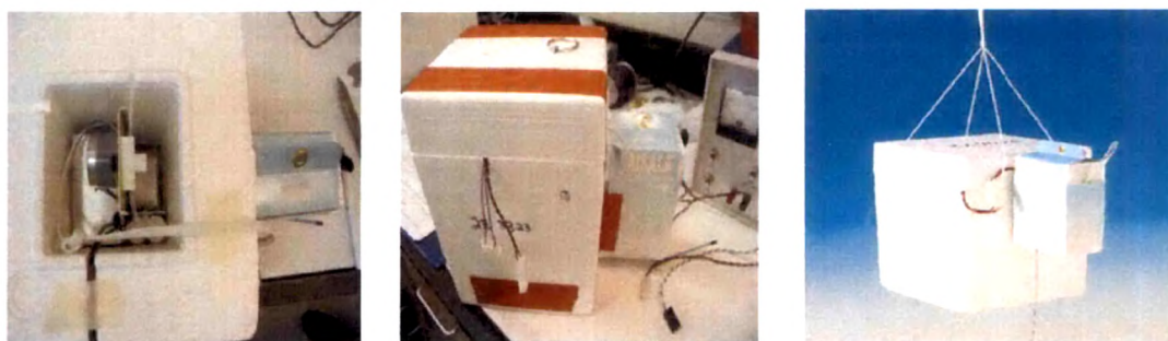
Figure 2.5. Ozonesensor in side the styrofoam box, (middle) a packed ozonesonde along with attached radiosonde (left). A combined unit of ozonesonde and radiosonde is ready for flight is shown on the right side (right).
