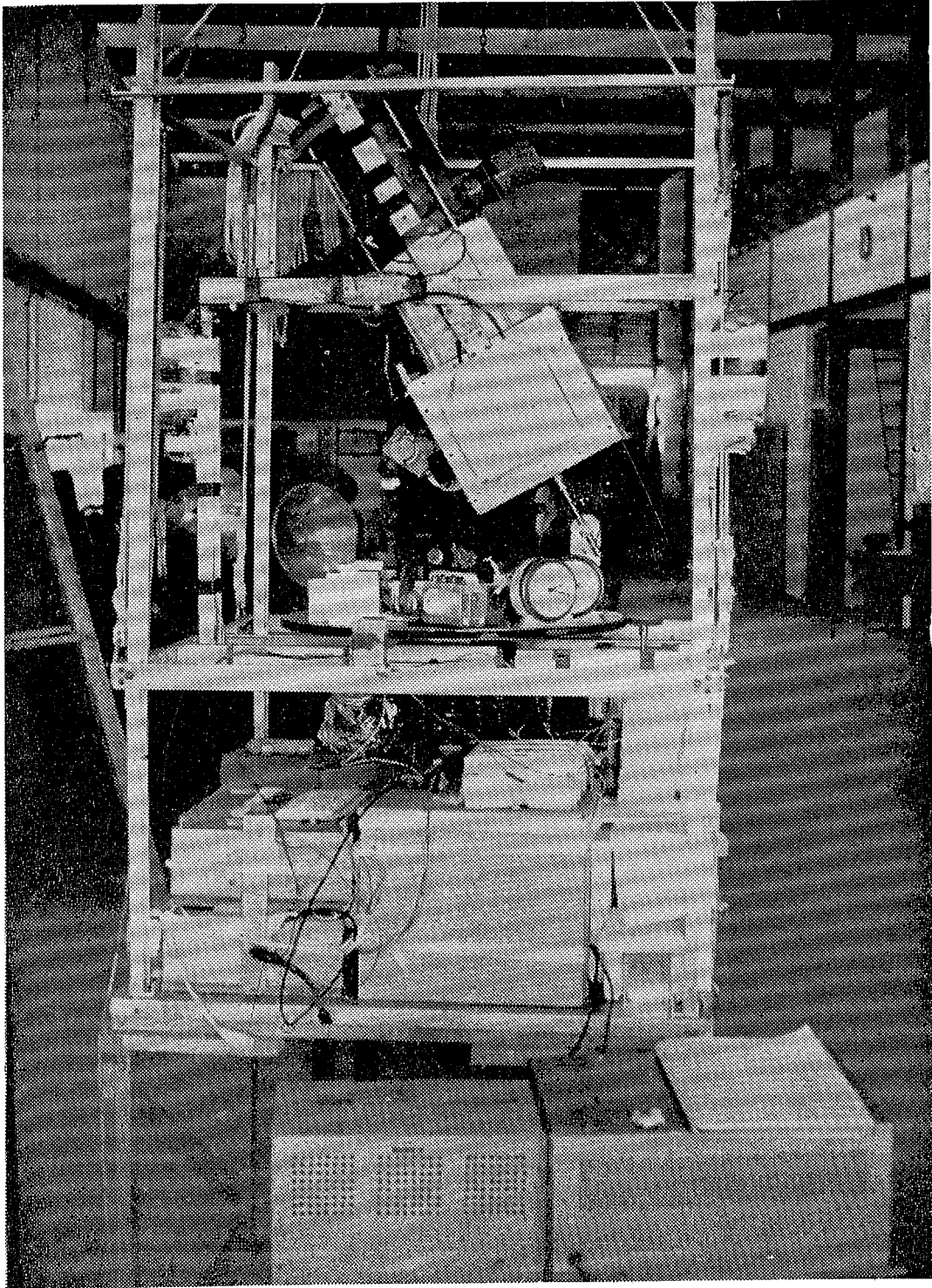
The picture shows the balloon payload before packing for launch. The clocks seen are used as timers for starting the tracking controls at proper times.
