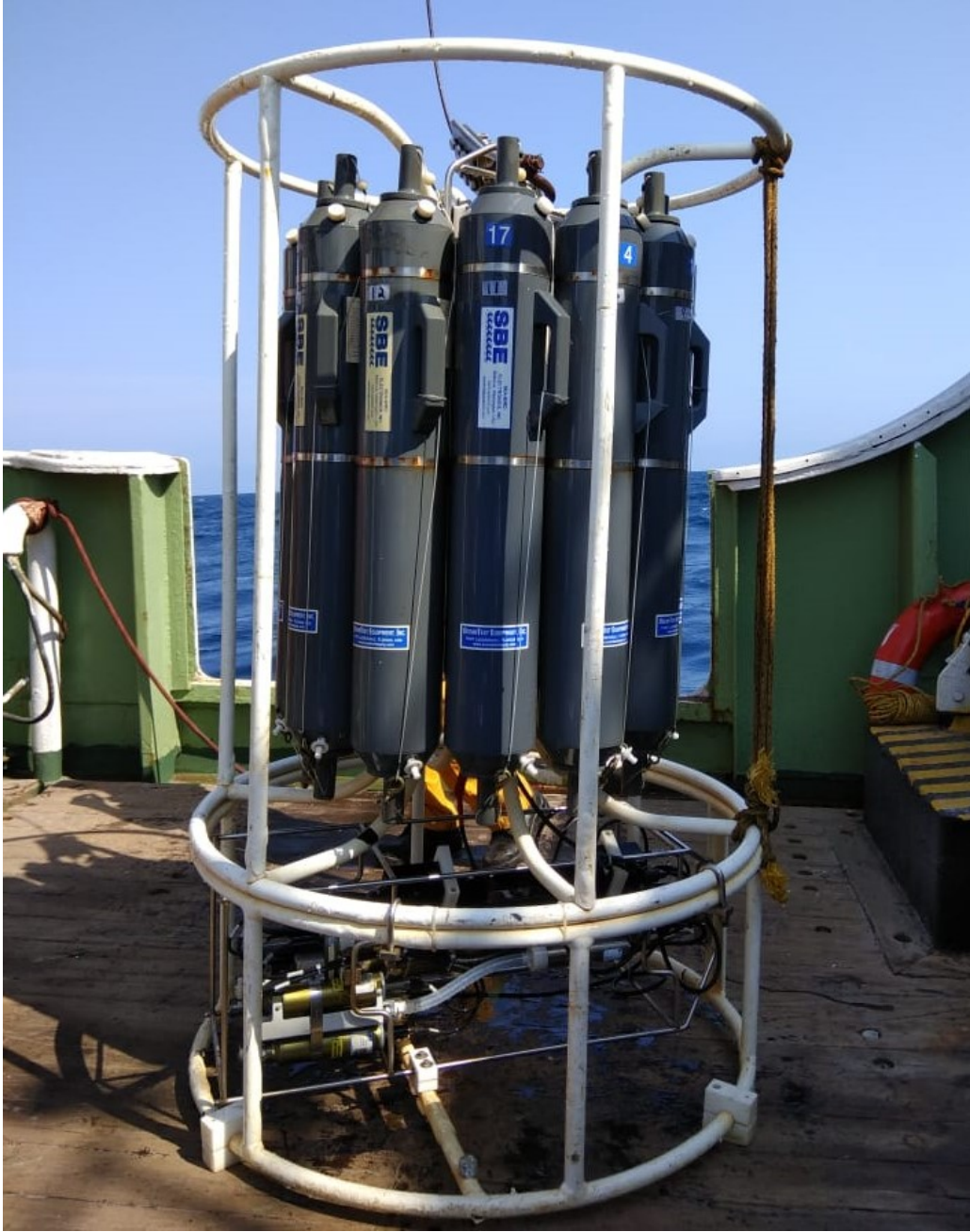
Figure 2.2: Niskin bottles and CTD, O 2 concentration, fluorescence and photosynthetically active radiation sensors mounted on the rosette sampler during the Sindhu Sankalp (SSK-127) cruise in the Bay of Bengal.
