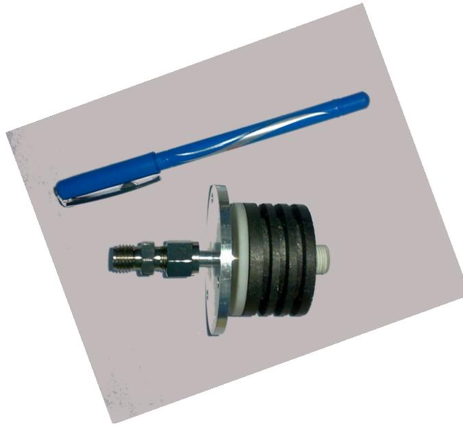
Figure 2.3: Photograph of the compact hollow cathode carbon cluster source.
