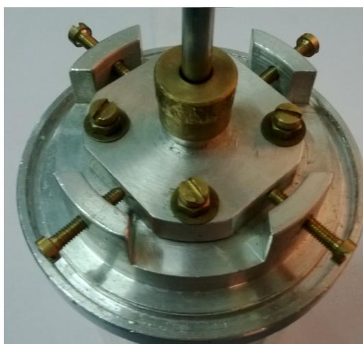
Figure 2.8: Top view of ISO-63 flange used for mounting pulsed nozzle and to adjust it in x, y direction during the operation.
