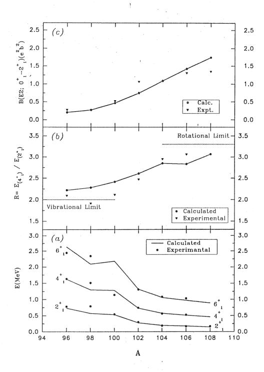
Figure 4.3: The experimental and calculated (a) Yrast spectrum; (b) Ratio of the energies of the  $4_1^+$  and  $2_1^+$  levels; and (c) The E2-transition probability  $(B(E2)\uparrow$ .
