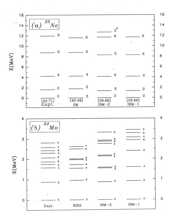
Figure 4.1: Comparison between IBM-1 and IBM-2 spectra of (a)<sup>20</sup>Ne and <sup>94</sup>Mo. The Experimental (Expt.) results for both, the Shell-Model (SM) spectrum for <sup>20</sup>Ne and BSDI (Chen et~al.~1986) spectrum for <sup>94</sup>Mo are also plotted.
