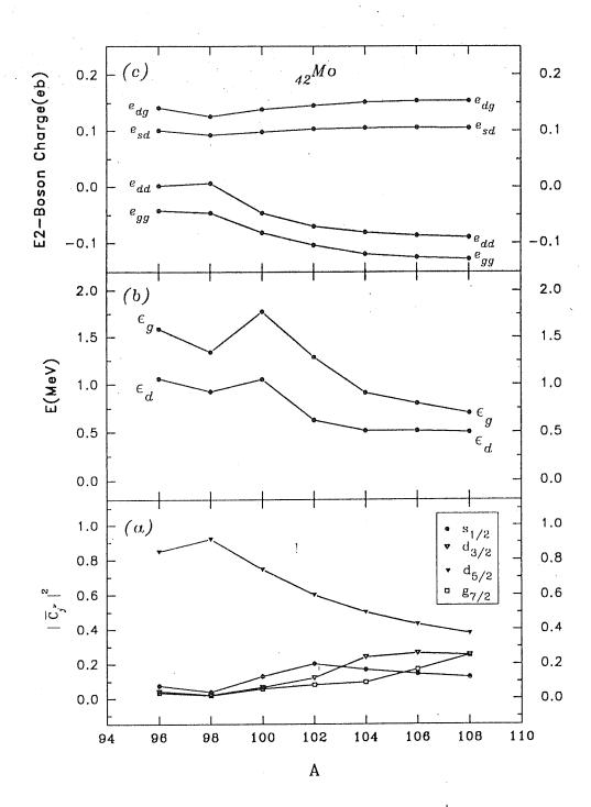
Figure 4.2: (a)Effective occupancies  $|\bar{C}_{j_i^{\nu}}|^2$  of s.p. neutron orbits from  $|\nu; k = +\frac{1}{2}\rangle_{\text{eff}}$  orbit; (b) The IBM-1 d- and g- boson energies  $\epsilon_d$  and  $\epsilon_g$  w.r.t.  $\epsilon_s$  and (c) The IBM-1 effective boson charges for E2-transitions are plotted against the atomic number A.
