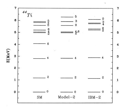
Figure 3.1: Spectrum of  $^{44}Ti$ . The plots labelled 'SM' and 'Model-2' are the Shell Model and (sdg)IBM-1 spectra of Skouras *et al.*(1990). The plot labelled 'IBM-2' is the spectrum generated by our scheme with s, d, g bosons.
