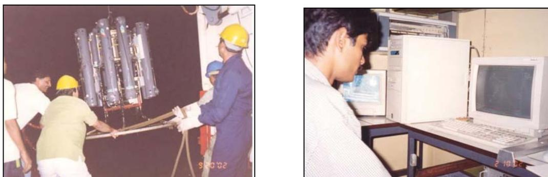
**Figure 2.2** Sampling of seawater onboard ORV Sagar Kanya. Left: Rosette attached with 30L Go-Flo bottles and underwater CTD unit being hauled up after temperature-salinity profiling and seawater sampling. Right: deck unit onboard for real time data acquisition and monitoring the sampling operation.
