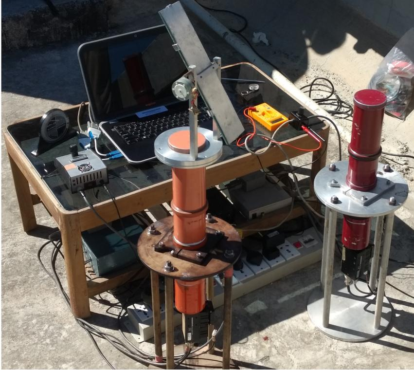
**Figure 2.1:** A typical field set up of the two portable narrow band and narrow field of view 630.0 nm airglow photometers. The red and orange colored photometers are operated in zenith and east mode, respectively.
