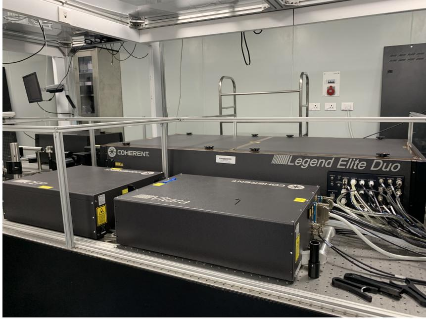
FIGURE 2.2: The femtosecond laser facility in PRL, Ahmedabad. It is a carrier-envelope phase stabilized Ti:sapphire laser (Coherent) producing 29 fs, 800 nm, linearly polarized pulses having intensity of the order of  $\sim 10^{12}$  W/cm<sup>2</sup> (average power of 10 W).
