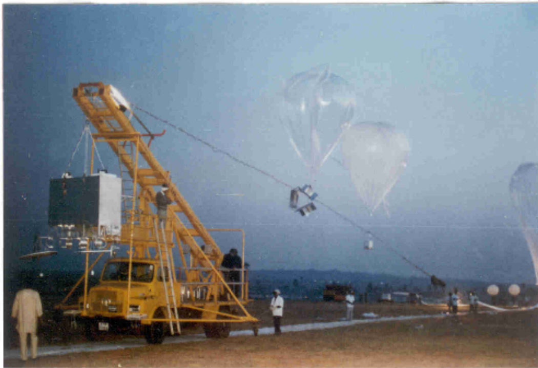
Figure 4.7: Picture showing the payload assembly on the launch truck, alongwith the radar target, radiosonde etc. and the launch balloon, minutes before the launch.
