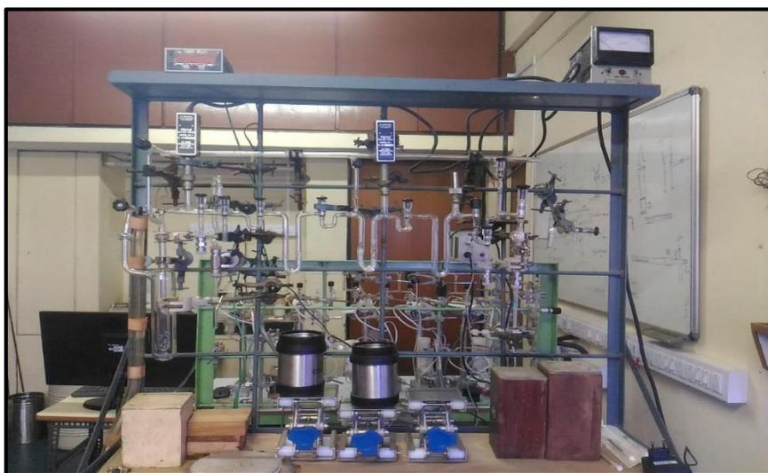
**Figure 2.10:** CO<sub>2</sub> preparation system for the carbonate type samples at Physical Research Laboratory, Ahmedabad.
