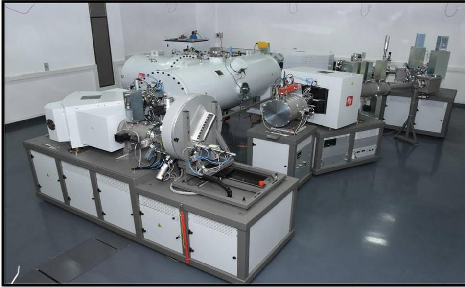
**Figure 2.11:** 1MV-AMS (HV make) installed at Physical Research Laboratory, Ahmedabad. Radiocarbon dating for sediment core samples used in this study was carried out using this instrument.
