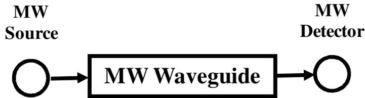
Figure 2.10: Block diagram of microwave water sensor.
