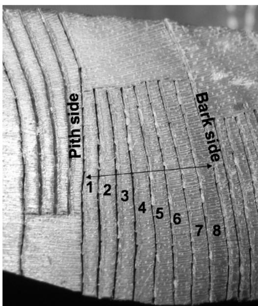
**Fig.2.9.** Photograph of a ring subdivided into 8 parts for studying sub-annual  $\delta^{18}\text{O}$  variations.
