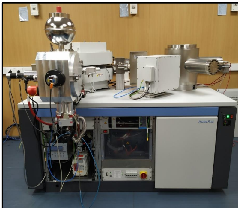
Fig. 3.6. Photograph of the Thermal Ionization Mass Spectrometer (Thermo® Triton Plus) used for analytical work.
