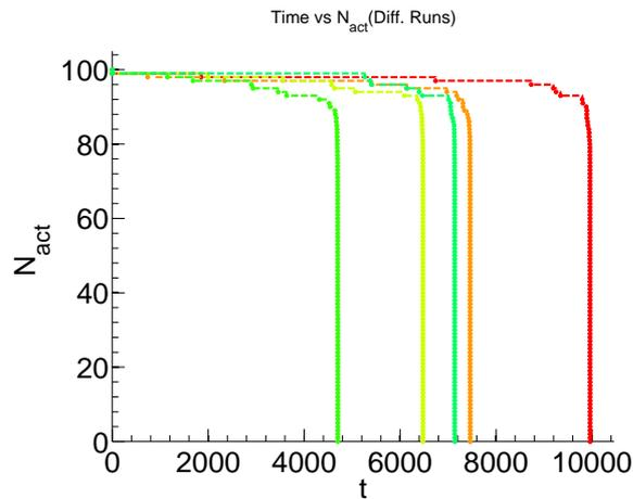
Figure 4.2: Number of active nodes on a network as a function of time. The capacity of each node is  $q = \langle f \rangle + 5\sigma$ . Different colors represents different initial conditions of walkers on the network. The simulation is performed on a fully connected network with  $N = 100$  nodes,  $E = 4950$  links and  $W = 2E$  walkers.
