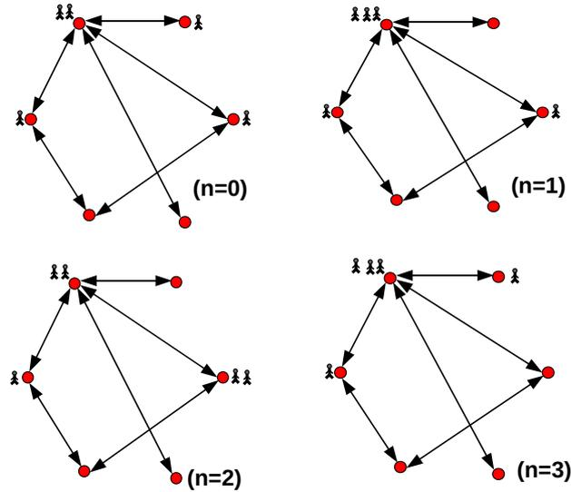
Figure 3.2: Random walk biased towards the hub ( $\alpha > 0$ ) is shown here using a schematic diagram. Walkers remain confined to the large degree nodes.
