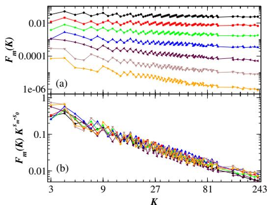
FIG. 2 (color online). Probability for occurrence of extreme events for several values of threshold  $q = \langle f \rangle + m\sigma$ . (a) shows the extreme event probabilities in log-log plot obtained from simulations with  $\Delta = 0$ . (b) shows scaling EE probabilities.  $S_0$  represents the reference slope with  $m = 2$ . The threshold applied for curves from top to bottom are  $m = 2.0, 2.5, 3.0, 3.5, 4.0, 4.5$ , and  $5.0$ .
