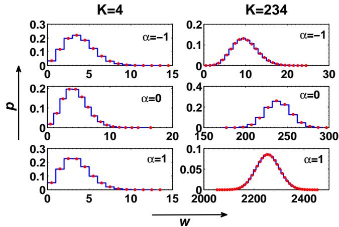
Figure 3.4: The distribution of walkers on two nodes with  $k = 4$  and  $k = 234$  for  $\alpha = -1.0, 0.0$  and  $1.0$ . The solid lines show the distribution of walkers obtained from simulation while the solid circles belong to the binomial distribution obtained analytically using the stationary probability in Eq. (3.7).
