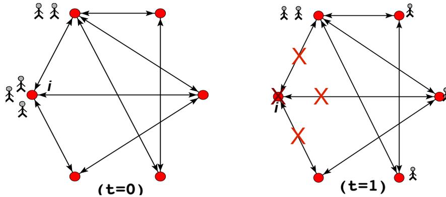
Figure 4.1: A network failure model is proposed based on extreme events. At  $t = 0$ , extreme event occurs at node  $i$  and it gets deleted from the network at the next time step i.e.  $t = 1$ . Before the node is deleted, walkers present on the node move to neighboring nodes as per the dynamical rules.
