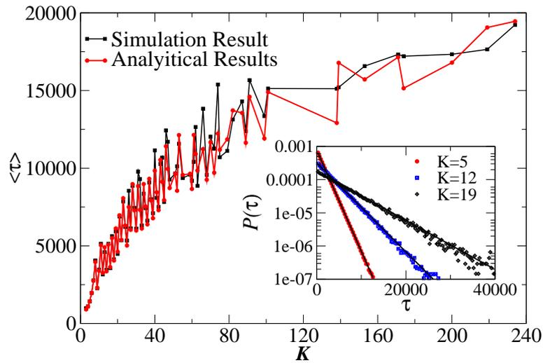
Figure 2.6: The inset shows the recurrence time distribution for extreme events from simulations (symbols) with  $\Delta = 0$  for nodes with 5, 12 and 19 links. The solid line is the analytical distribution. The main figure shows the mean recurrence time as a function of degree  $K$ .
