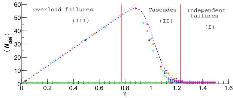
Figure 4.6: The number of deleted nodes are plotted against the capacity-load ratio. Blue dashed line is obtained from Eq. (4.15). Symbols represent the data obtained from simulations. Different symbols are used for different realizations. Along the black dot-dash line,  $\langle N_{del} \rangle = N_{act}$ . Red solid lines are used for separating the different natures of failure. Along the green solid line  $\langle N_{del} \rangle = 1$ .
