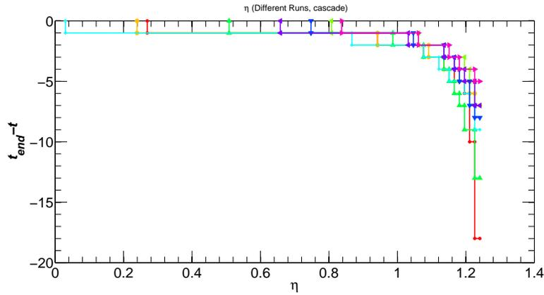
Figure 4.8: The time at which a node fails is plotted as a function of the capacity-load ratio in the region of cascade failures and over load failures ( $0 < \eta < 1.25$ ). Here, the time of the total failure is considered as 0 and '-' sign represents the time steps just before the network failure. Again, different colors are used for different realizations.
