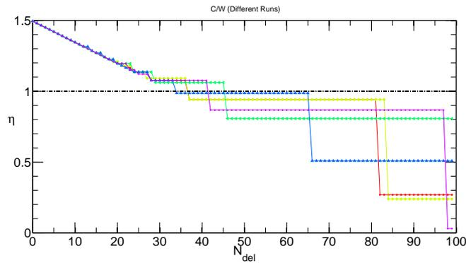
Figure 4.5: The ratio  $\eta = C/W$  is plotted against the number of deleted nodes in the network. Different colors represent different realizations. On the black dash-dot line the capacity of the network equals the total load(walkers) on the network.
