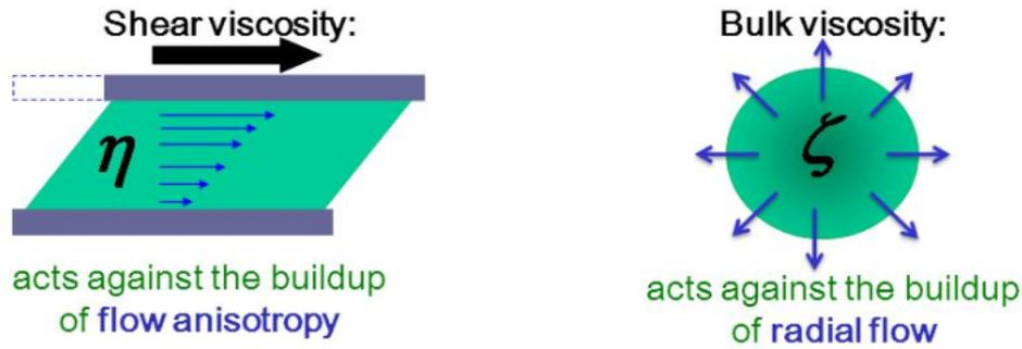
Figure 1.3: Origin of shear and bulk viscosities.
