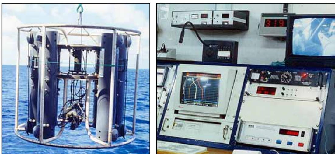
*Figure 2-5 Sampling of seawater onboard FORV Sagar Sampada. Left: Rosette attached with eight 30lit Go-Flo bottles and SBE 9 underwater CTD unit being lowered for temperature - salinity profiling and seawater sampling. Right: The SBE 11 deck unit onboard, for data acquisition and monitoring the sampling operation. Real time profiles of temperature (red), salinity (blue), oxygen (green) and beam attenuation (brown) can be seen on the monitor.*
