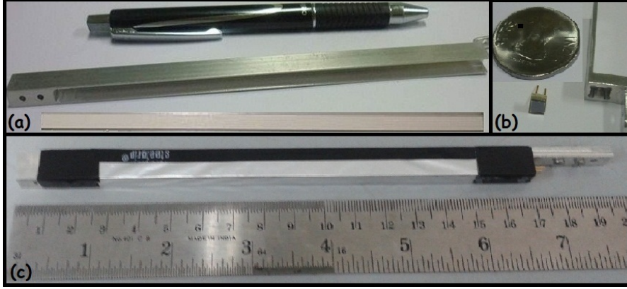
Figure 3.15: (a) A CsI(Tl) scintillator ( 5 \text{ mm} \times 5 \text{ mm} \times 150 \text{ mm} ) and its aluminium holder. (b) A Si photomultiplier ( 3 \text{ mm} \times 3 \text{ mm} ) with its aluminium case. (c) The complete CsI(Tl)-SiPM package. The CsI(Tl) is coupled to the SiPM using optical glue and wrapped by a thin aluminium foil for light tightness. 16 such CsI(Tl)-SiPM systems have been used in the final Compton polarimeter configuration
