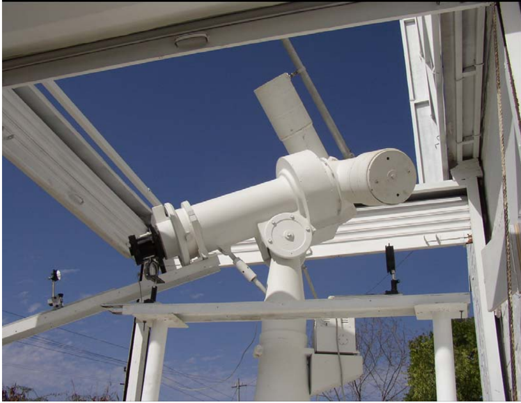
Figure 3.1: 15 cm Zeiss Coudé Telescope being used as the light feed for prototype adaptive optics at USO. In addition to the telescope, a 50 mm diameter mirror and two 150 mm diameter doublets used for relaying the primary image to inside the laboratory are also shown. The telescope, supporting optical benches, shelter and side wall of the building are all painted with matt finish white paint rich in \text{TiO}_2 so as to maintain the surfaces close to the ambient air temperature.
