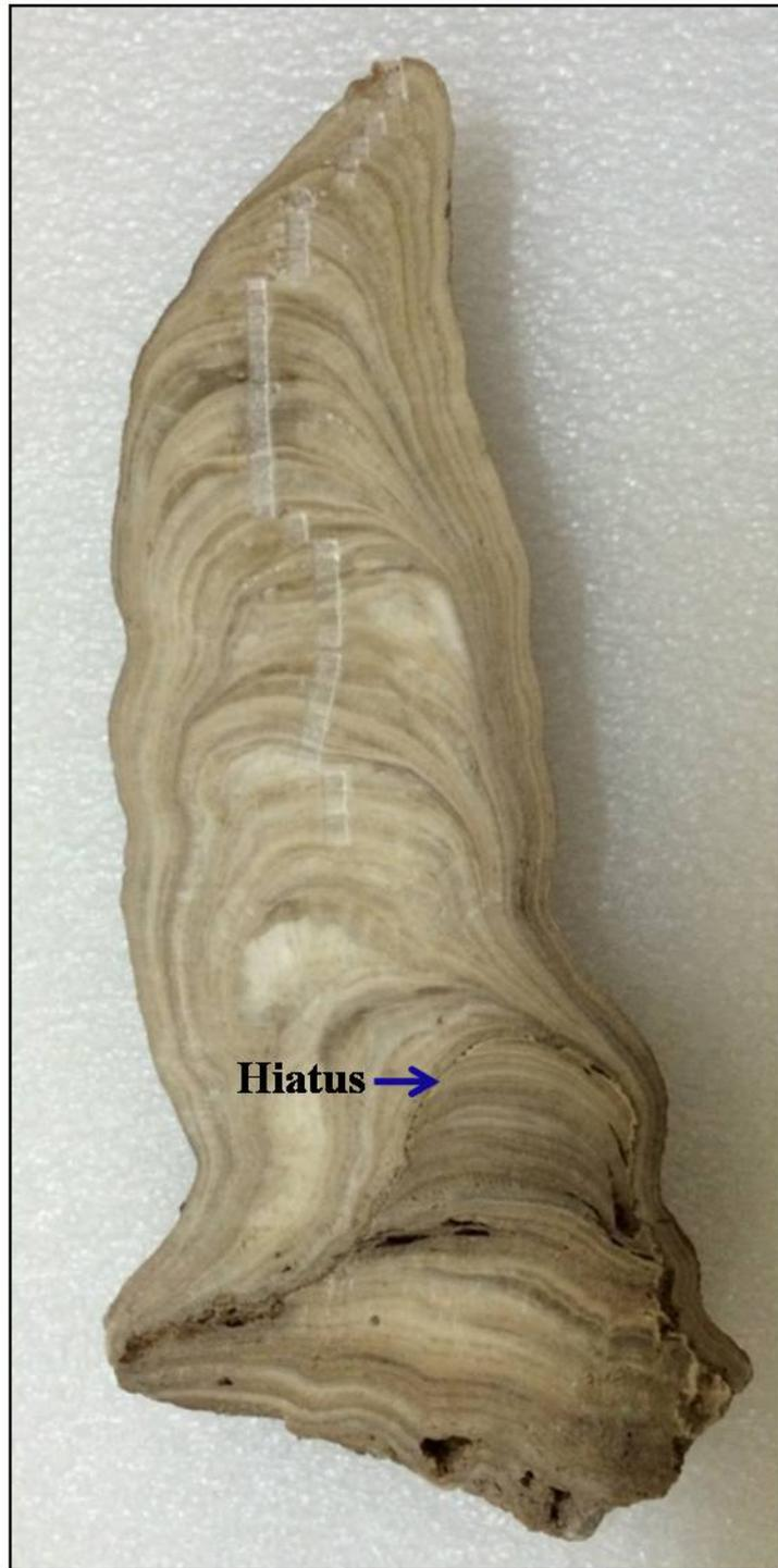
**Figure 3.3:** *Polished cross sectional view of the Dandak-I stalagmite. Planar view of the growth layers indicated constant shift in the drip direction, changing the growth axes. Near the bottom, a hiatus (Blue arrow) is observed as a distinct boundary separating two growth phases. Post hiatus, the growth axis has shifted and there is a continuous growth thereafter.*
