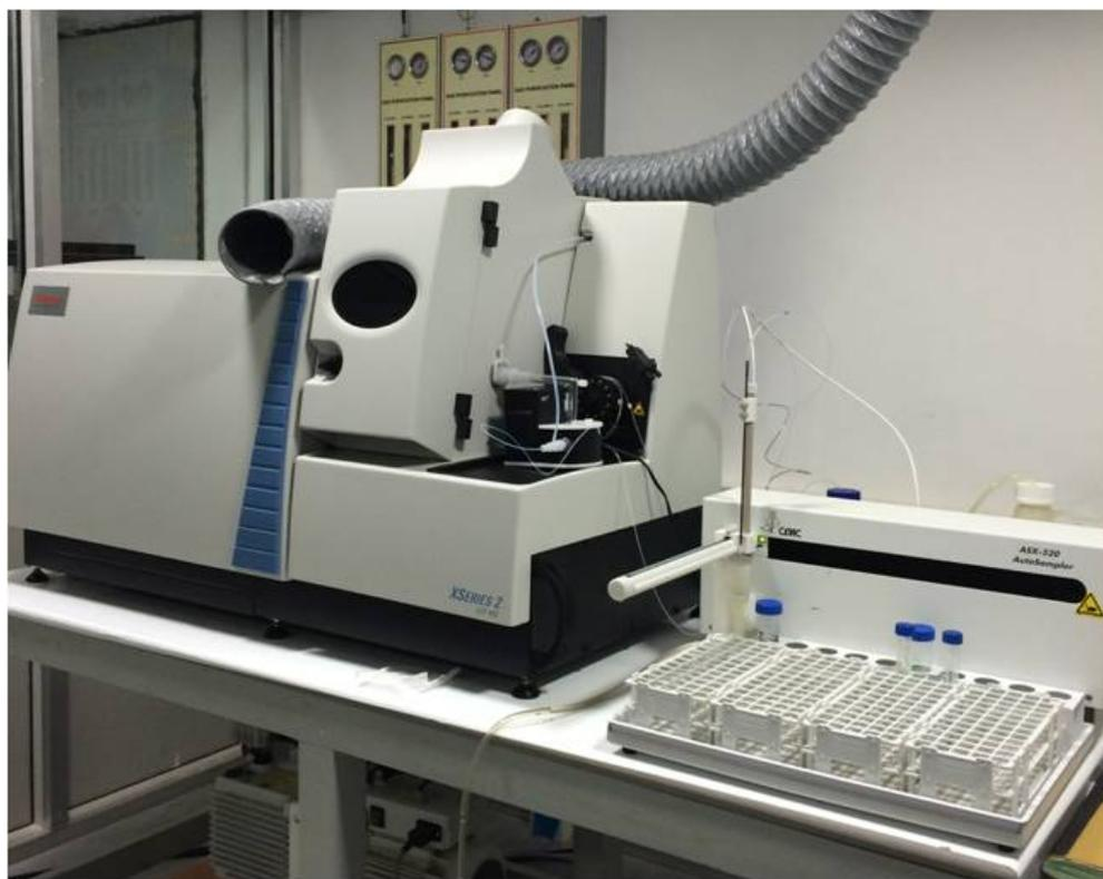
**Figure 3.14:** *Thermo-scientific Quadrupole-Inductively Coupled Plasma mass spectrometer at PRL, Ahmedabad.*
