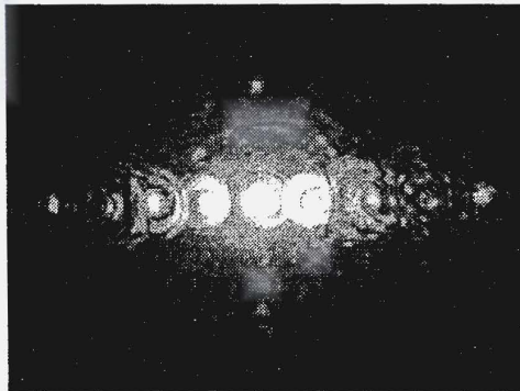
Figure 2.14: Bessel beam of zeroth order produced in the 1st order diffraction pattern.
