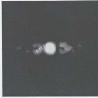
Figure 2.4: Horizontal Gaussian vortex diffracted orders for white coherent light fall on fork grating.
