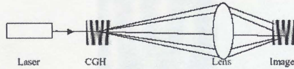
Figure 6.1: Experimental set up for Imaging of scatterer by interfering transmitted diffracted orders
