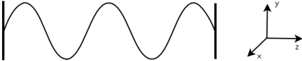
Figure 1.1: Single mode radiation field, considered as equivalent to a quantum harmonic oscillator, within a one-dimensional cavity oriented along z-axis.
