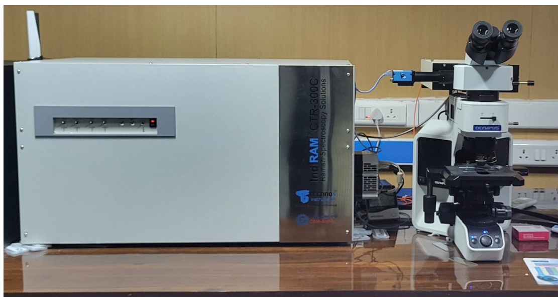
Fig. 2.9: IndiRam CTR 300C micro-Raman spectrometer coupled with an Olympus BXM-53M microscope at the Physical Research Laboratory (PRL), Ahmedabad, India
