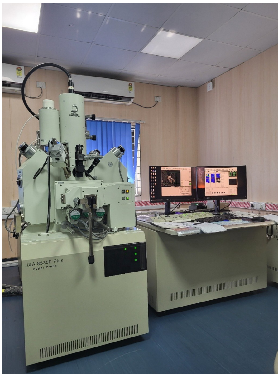
Fig. 2.7: Image of the Field Emission Electron Probe Microanalyzer (FE-EPMA) facility at the Physical Research Laboratory (PRL), Ahmedabad, India
