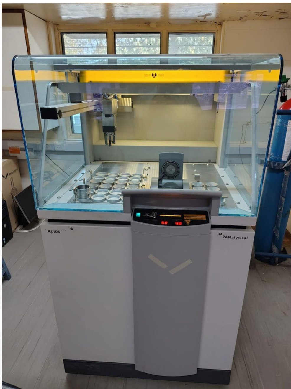
Fig. 2.10: Image of the Philips AXIOS X-ray fluorescence (XRF) spectrometer with a rhodium (Rh)X-ray tube, housed at the Physical Research Laboratory (PRL), Ahmedabad
