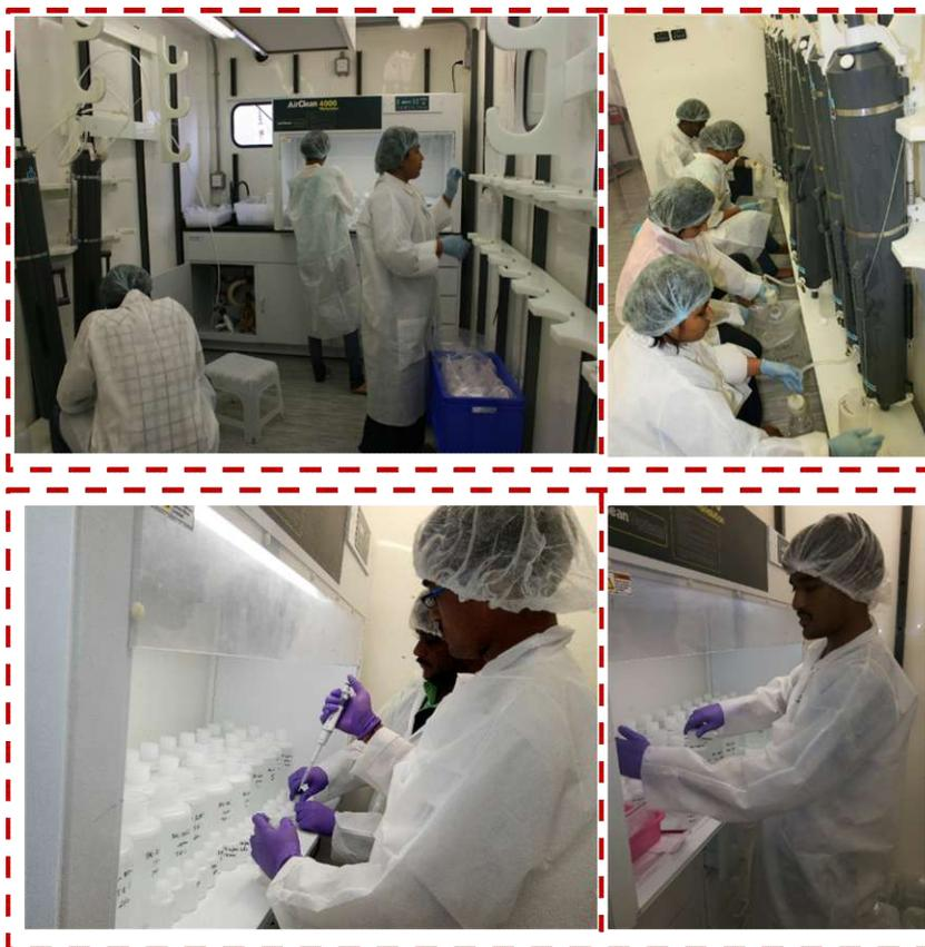
**Figure 2.6:** Seawater filtration, collection, acidifying and packing onboard ORV Sagar Kanya.
