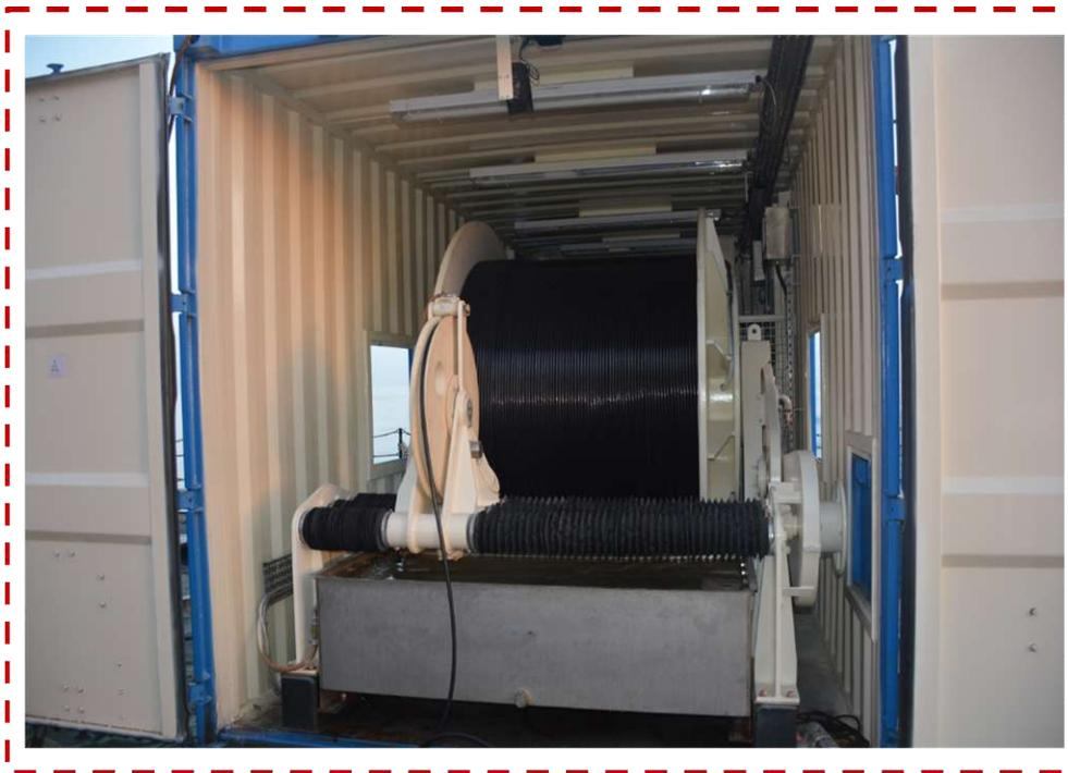
**Figure 2.4:** Winch van containing 8000 m long Kevlar cable.
