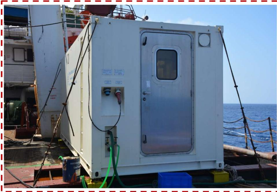
**Figure 2.5:** Class-1000 clean van on board ORV Sagar Kanya for sub sampling of the seawater.
