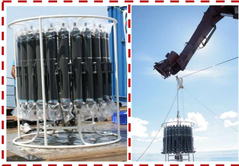
**Figure 2.3:** Trace metal CTD with 24 x 12 L Niskin bottles mounted on an aluminum powdered rosette (Left), CTD frame connected to a Kevlar cable through a Teflon pulley (Right).
