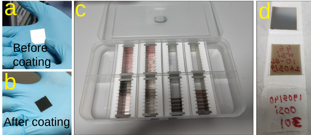
Figure 6.12: Panels a and b show the image of a substrate before coating and after coating respectively. Panel c : a set of single-layer mirrors coated with different thicknesses of Si or W. Panel d : Zoom view of three mirror foils. At the backside of each foil, a unique id is given corresponding to the sputtering parameters.
