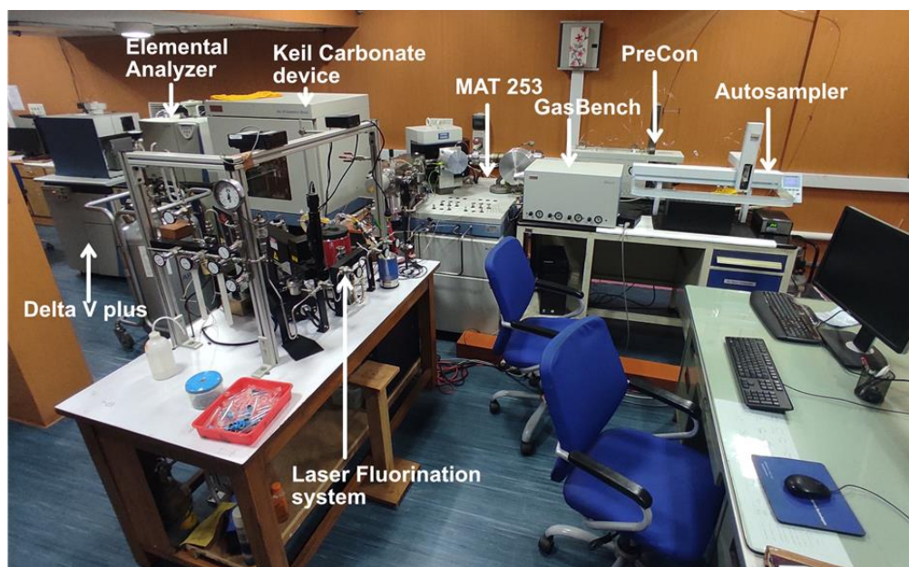
Figure 2.3 Photograph of the Geosciences-Stable Isotope Laboratory (GeoSIL), Physical Research Laboratory, Ahmedabad, India. Name of the available facilities in the GeoSIL are marked in the photograph.
