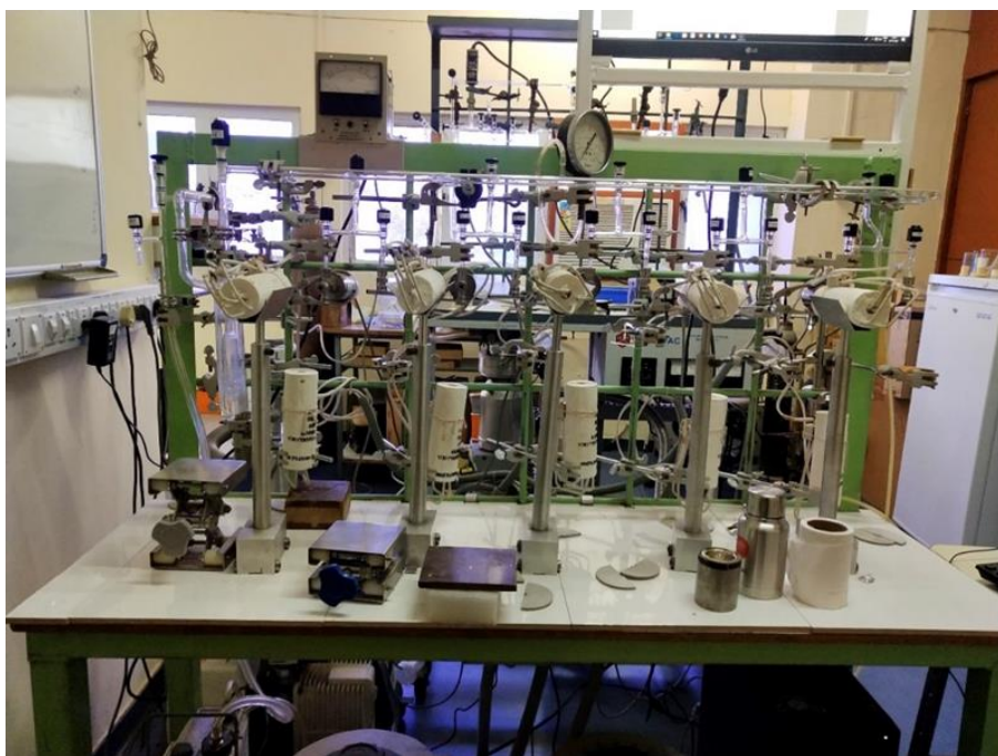
Figure 2.7 Graphitization system for extracted CO 2 at the Radiocarbon Laboratory, Physical Research Laboratory, Ahmedabad, India.
