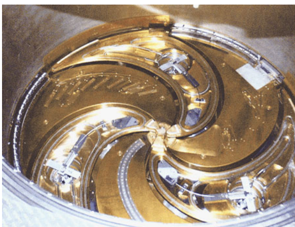
Fig. 16.7 View into the spiral-shaped superconducting polefaces of the LNS SC cyclotron, that have a diameter of 1.8 m, magnetic fields between 2.2–4.8 T, accelerating fully stripped light ions such as ^{12}\text{C} up to 80 MeV/u
