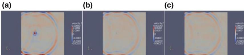
**Fig. 6.22** Distribution of Z velocity vector components on the upper surface for 300 time step: **a** intact material, **b** delamination area 2 mm, **c** delamination area 4 mm
