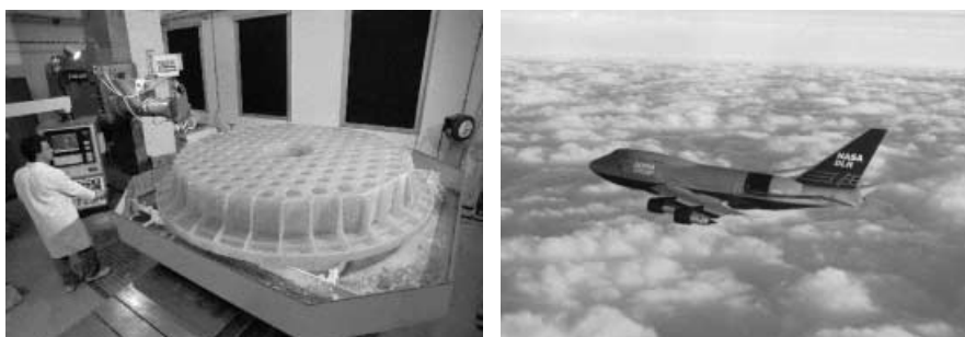
Fig. 1. Left: The SOFIA primary mirror is now light weighted by 80 % and is being polished at REOSC in France. Right: The SOFIA 747-SP aircraft, originally dedicated as the 'Clipper Lindbergh'.
