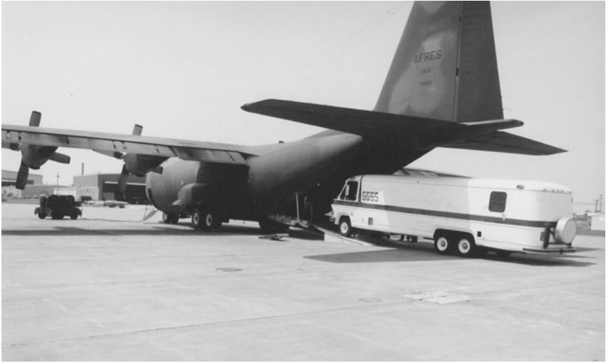
Fig. 11.1 A different approach to airborne installation. The camper-van containing the US Air Force prototype gradiometer being driven into a C130 for a test flight in 1987. Jekeli (1988) noted that amongst the equipment required was 'optionally a reporter for Ripley's Believe-It-Or-Not'. Photo provided by Christopher Jekeli
