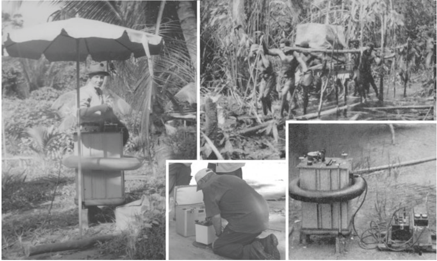
Fig. 9.6 The LaCoste gravity meter in action. Anti-clockwise from the bottom right. 1 An early model LaCoste meter, as used in APC-IEC surveys in Papua in the late 1930s. 2 The meter being transported through the Papuan swamps. 3 The meter set up ready for a reading. 4 The modern equivalent. Photos, except for (4), courtesy of Oilsearch Ltd
