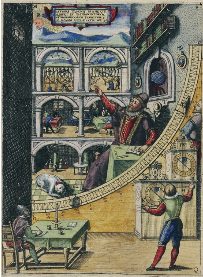
Fig. 3.8 The great mural quadrant in Uraniborg, from the 1602 edition of Astronomia Instauratae Mechanica . The graduated scale, a form of transversal that allowed angles to be measured to better than a minute of arc without the need for the accurately engraved 90^\circ arcs used in earlier and smaller instruments, was mounted on a wall oriented very precisely N-S. The accompanying text gives the radius of the arc as 5 cubits, or about 3 m, which suggests that it and Tycho (who is pointing to the small window through which the observations were made) are drawn to approximately the same scale, dwarfing his helpers and assistants. Even the observer making the measurements, although almost Tycho-size, is squashed in against the right-hand edge of the picture. The dog at Tycho's feet may be one of the pair of English mastiffs presented to him by the future James I of England (VI of Scotland)
