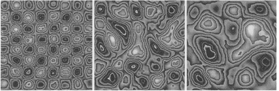
Fig. 3: Examples of calculated vorticity fields, showing the qualitative evolution of the flow from a large number of small vortices, to a smaller number of larger vortices. The overall exponential decline of the energy does not allow the final state to be reached. Left: t^* = 0 s (initial field). Middle: t^* = 4.2 s. Right: t^* = 11 s.
