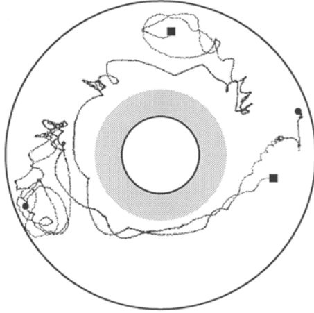
Fig. 5. Two trajectories show the lack of long-lived coherent structures in the weakly turbulent flow . The beginning and end of one trajectory is marked with circles, the other with squares; both particles start at the far right. The inner and outer circles represent the annulus boundaries, and the grey circle indicates the location of the Plexiglas barrier. The particles are shown in the reference frame of the annulus. (Figure based on Ref. [11].)
