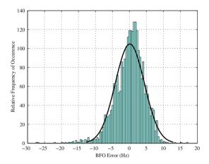
to be conservative and allow for potential variation in the  $\delta f_k^{\text{bias}}(\mathbf{x}_k,\mathbf{s}_k)$  value on the accident flight, our model assumes a noise standard deviation of 7 Hz. Section 5.5 illustrates the sensitivity of the BTO and BFO measurements to variations in the aircraft state.
