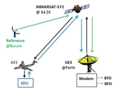
Fig. 5.1 System model of the satellite communication system
