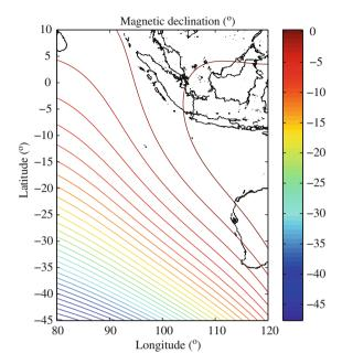
the Indian Ocean region. There are significant variations in magnetic declination in the areas through which the accident flight is thought to have flown. If the aircraft had been following a fixed compass reading then it would appear to gradually turn. Each of the different autopilot modes is now briefly described.
