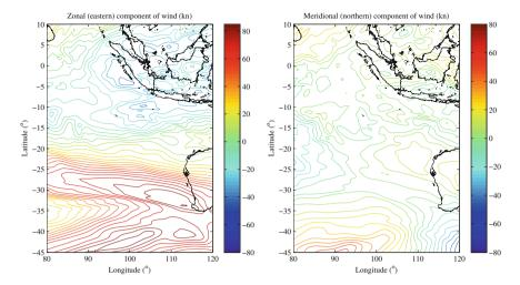
**Fig. 6.3** Wind data for 8 March 2014, 00:00, at 175 hPa (approximately 41,000 ft). Contour lines are drawn every 5 kn. The zonal component of the wind is the component blowing toward the East, while the meridional component is the component blowing toward the North
