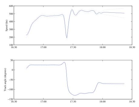
**Fig. 4.2** Smoothed estimates of speed and direction derived from radar data. *Dotted lines* show covariance of estimates, illustrated as mean plus and minus three-sigma value
