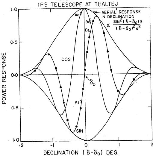
Fig. 1 Receiver fringes of correlation interferometer of radio telescope at Thaltej. A<sub>c</sub>, B<sub>c</sub> and A<sub>s</sub>, B<sub>s</sub> are assumed positions of 3C 298 on COS and SIN fringes.
