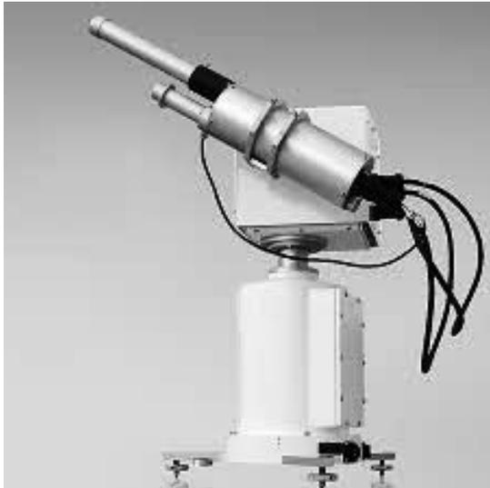
**Figure 1.** POM-01 Sky radiometer from Prede Co. Ltd., Japan
