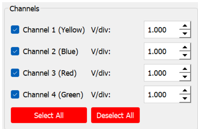
Figure 8. Checkbox option for enabling/disabling and V/div option for scaling individual channels
