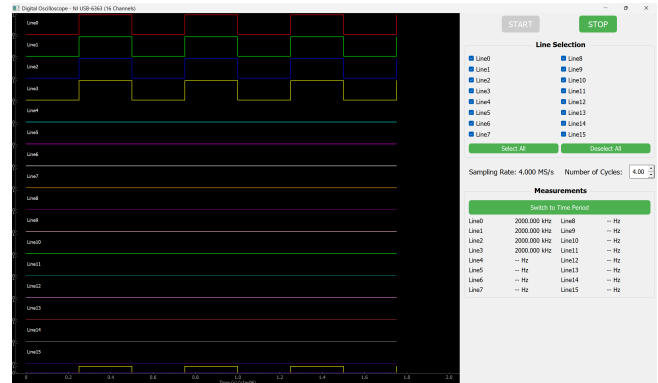
Figure 15. Digital read GUI showing 16-channel frequency measurement at 2MHz
