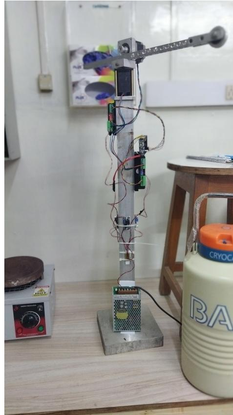
**Figure 9.** The Automated Freeze-Thaw instrument, after configured mechanically and electronically
