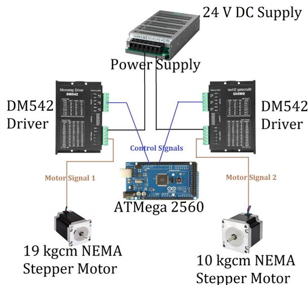
**Figure 4.** Schematic diagram representing the electronic controls of motors, including the three main components: power supply, motor drivers and the microcontroller
