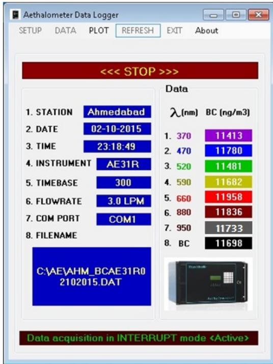
**Figure 5.** Aethalometer data screen during data acquisition operation
