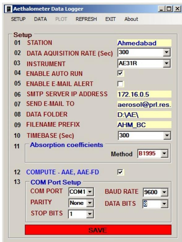
Figure 4. Setup configuration for Aethalometer data logger
