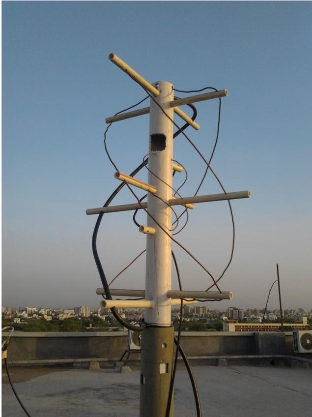
**Figure 2.** Photograph of the Quadrifilar Helix antennae for 150 MHz and 400 MHz (nested inside).
